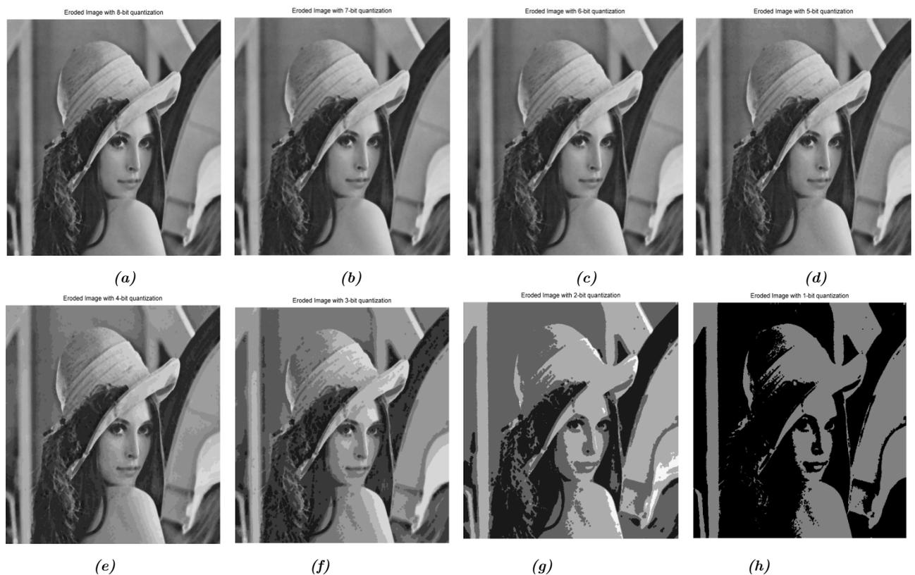
*Fig. 3.7 Bitwise erosion for several levels of bit quantization.*
