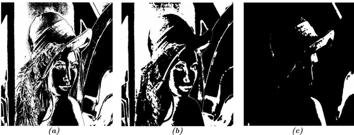
Fig. 3.2 (a) Original  $2^{\text{nd}}$  bitplane. (b) Erosion of the MCD branch ( $\mathcal{R}_2^1$ ) (c) Erosion of the NCD branch ( $\mathcal{S}_2^1$ ).
