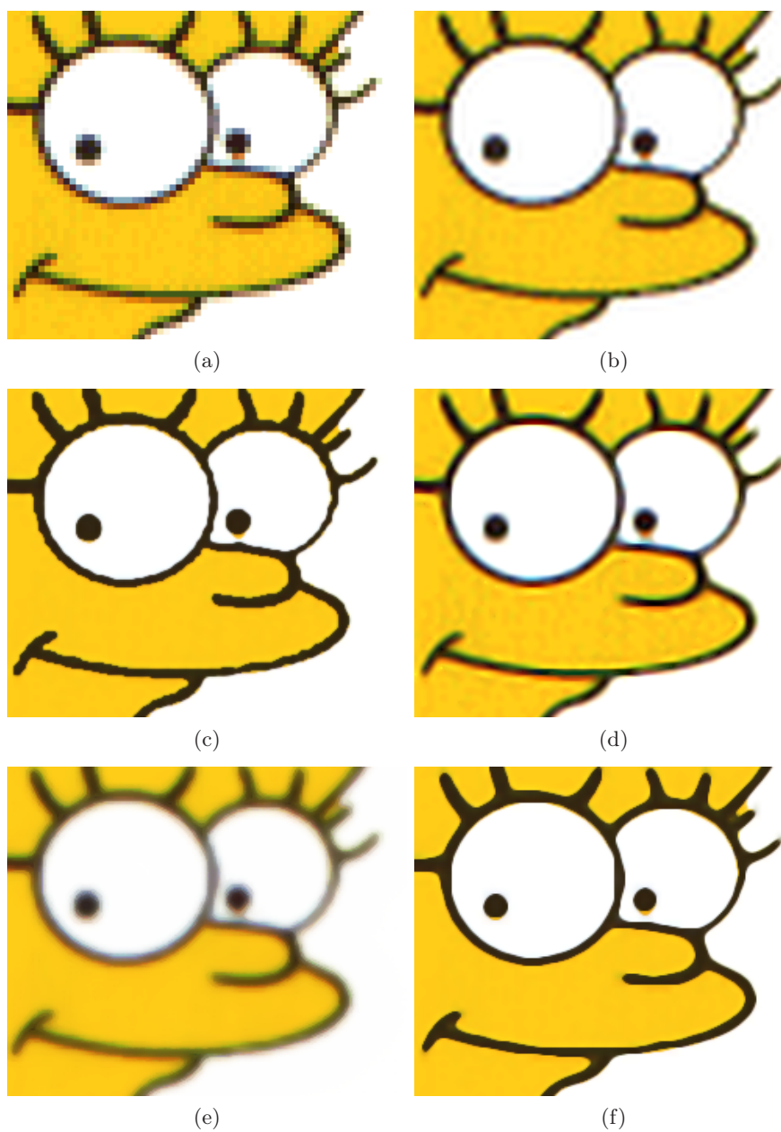
Figure 4.15: Restoration results of Lisa : (a) nearest neighbour, (b) cubic B-spline, (c) restoration with isotropic smoothing and multimodal colour priors, (d) restoration using geometry-driven smoothing without multimodal colour priors, (e) curvature preserving PDE's [Tschumperlé, 2006] and (f) proposed method.
