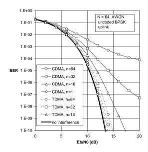
Fig.3 : Uplink BER performance for uncoded transmission over AWGN channel
