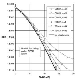
Fig. 5 : Uplink BER performance for coded transmission over flat Rayleigh fading channel
