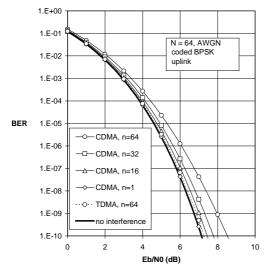
Fig. 4 : Uplink BER performance for coded transmission over AWGN channel
