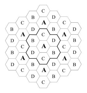
Fig. 1 : Cell structure for frequency reuse factor of 4.
