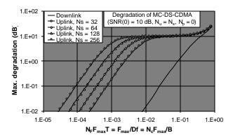
Figure 4: Maximum degradation caused by carrier frequency offset
