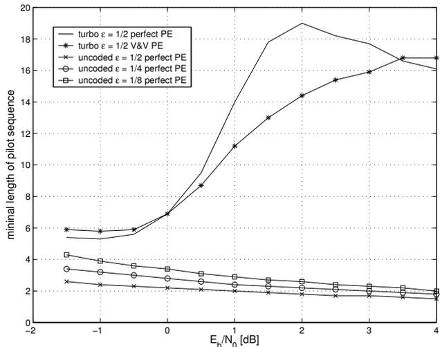
Fig. 2. Minimal length ( $L$ ) of pilot sequence for uncoded and turbo coded QPSK (for perfect phase estimation (PE) and a NDA PE algorithm from [1]).
