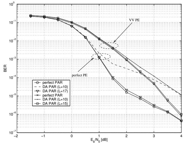
Fig. 3. BER performance for turbo coded QPSK for different values of  $L$  (for perfect phase estimation (PE) and a NDA PE algorithm from [1]).
