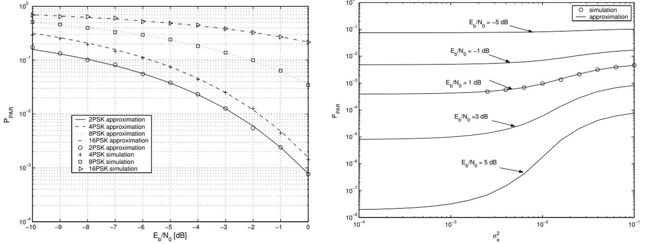
Fig. 1.  $P_{par}$  as a function of the SNR for a pilot sequence of 5 symbols for perfect phase estimation (left) and for Gaussian distributed phase errors (for 4PSK; right)
