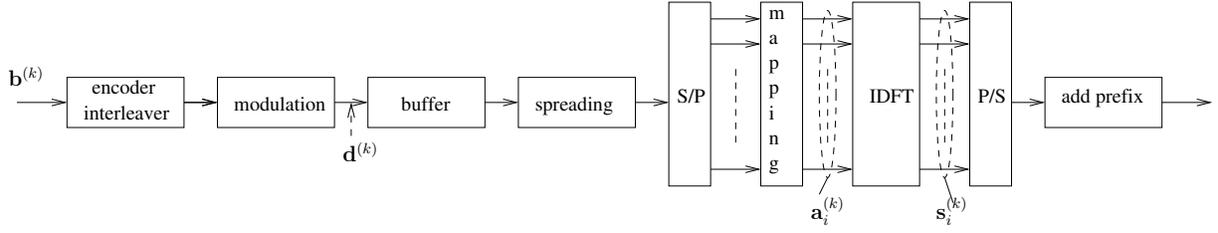
Fig. 1. Frame construction for the  $k$ -th user.
