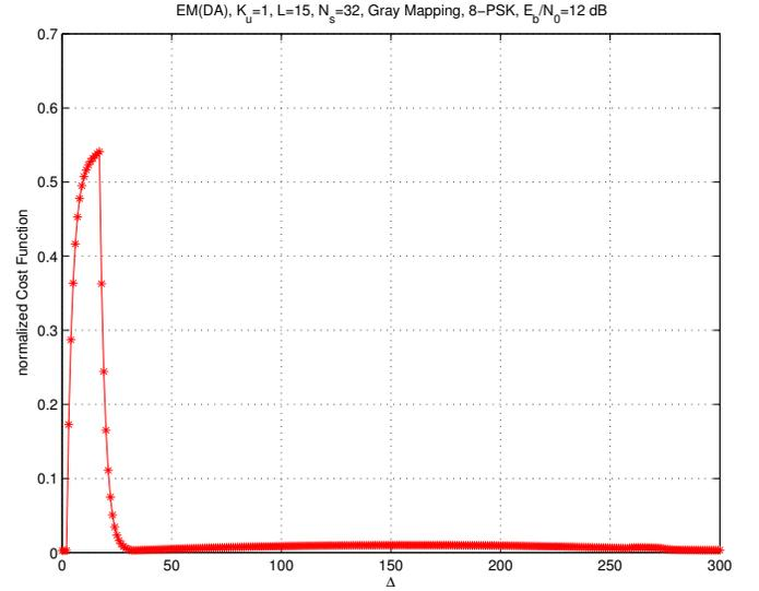
Fig. 2. DA frame synchronization: trial value of  $\Delta$  vs. cost function.  $\Delta$  equals 17.
