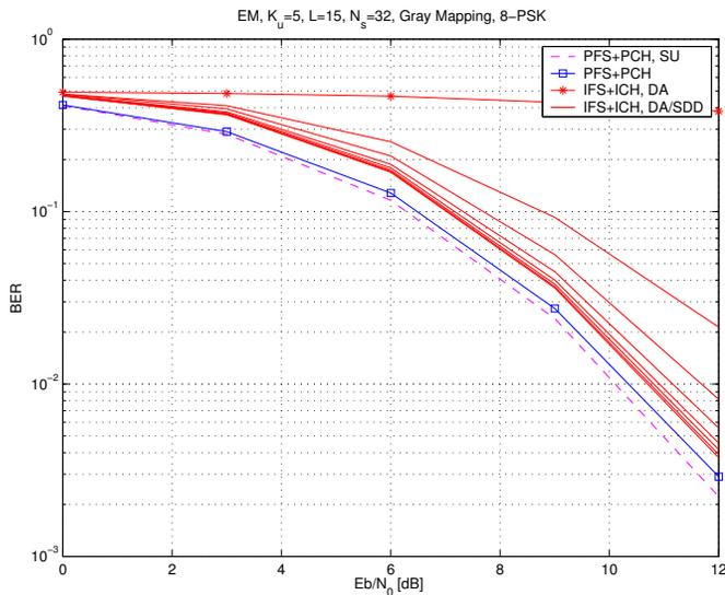
Fig. 4. Joint frame synchronization and channel estimation: BER performance
