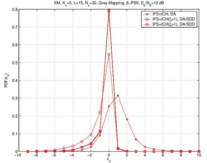
Fig. 3. Frame synchronization: pmf of estimation error at 12 dB
