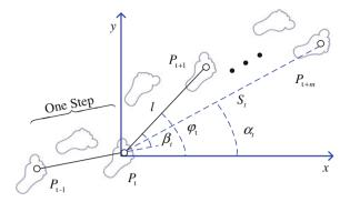
$$\begin{cases} x_{t+k,\text{PDR}} = x_{t,\text{WiFi}} + \sum_{i=1}^{k} l \cos \varphi_{t+k-1} \\ y_{t+k,\text{PDR}} = y_{t,\text{WiFi}} + \sum_{i=1}^{k} l \sin \varphi_{t+k-1} \end{cases}, \ k = 1, 2, \dots, m \tag{63.1}$$
