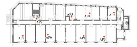
Fig. 63.4 Floor Plan of the indoor environment and the distribution of the APs
