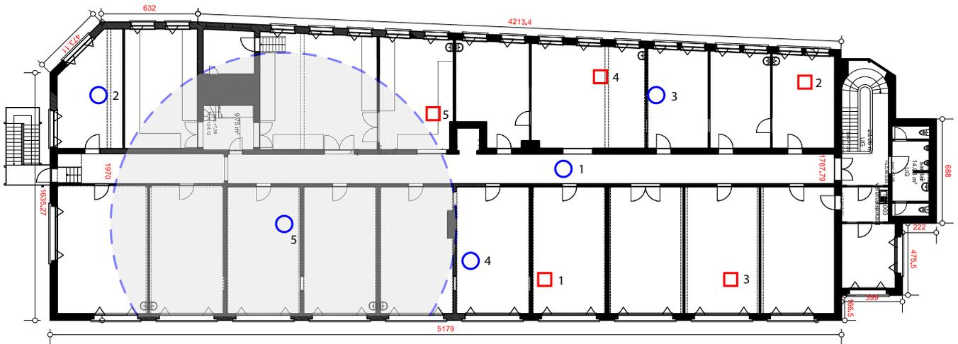
Figure 3. Floor plan of the office corridor in the university building used to model the 3D environment for ray tracing. The squares and circles represent the access points and anchors, respectively. For the fifth anchor, the radio range of 20m is shown. The access points have radio range within the entire corridor. The total area is over 900m<sup>2</sup>.
