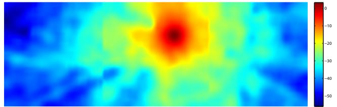
Figure 1. Radio map of a WiFi access point, generated by 3D ray tracing. The transmit power of the access point is 100mW. The signal strength values are given in dBm.
