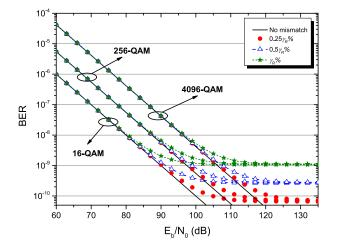
Fig. 7. Analytical BER curves in a Rayleigh channel for N = 2048, L = 8,  $\sigma_{TT}^2 = 0$ , different modulation type and mismatch levels.
