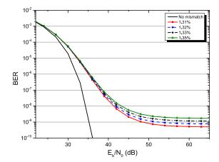
Fig. 5. Analytical BER curves in a wired channel for 16-QAM, N = 2048, L = 8,  $\sigma_U^2 = 0$  and different mismatch levels.
