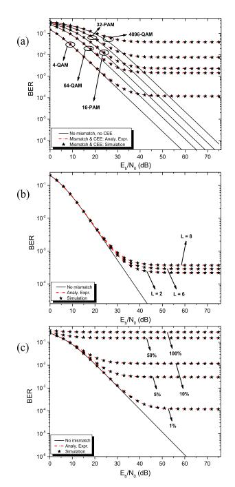
Fig. 2. BER curves for a Rayleigh channel with N = 2048. (a) L = 8, 1% mismatch and  $\sigma_U^2 = 10^{-4}$  for square QAM and PAM. (b) 16-QAM, 2% mismatch level and no CEE when L equals 2, 6 and 8. (c) 8-PAM, L = 7 and no CEE with different mismatch levels.
