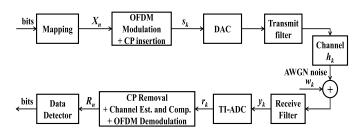
Fig. 1. Block diagram of an OFDM system with a TI-ADC at the receiver.
