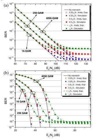
Fig. 8. BER curves for 16-QAM with  $BER_t = 10^{-9}$ , N = 2048, L = 8,  $\sigma_U^2 = 0$ , different mismatch level and  $5 \times 10^3$  sets of L random gain errors: (a) a Rayleigh channel, (b) a wired channel.
