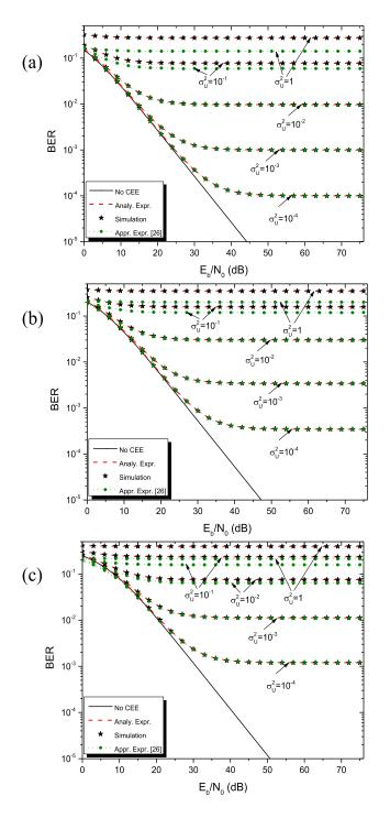
Fig. 3. BER curves for a Rayleigh fading channel for N = 2048, L = 8 and 0% gain mismatch with different values of CEE variance: (a) 4-QAM, (b) 16-QAM and (c) 64-QAM.
