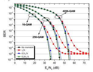
Fig. 6. Analytical BER curves in a wired channel for N = 2048, L = 8,  $\sigma_U^2 = 0$ , different modulation orders and mismatch levels.
