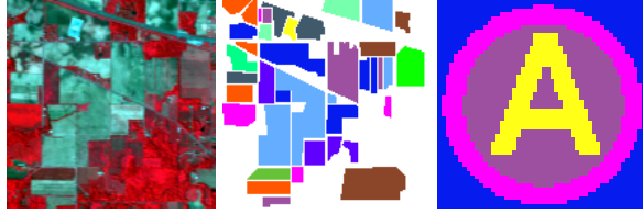
Fig. 3: HSI data sets used in our experiments. Left: false color image of Indian Pines; middle: ground truth; right: simulated HSI using the average spectral reflection of same class in the ground truth.
