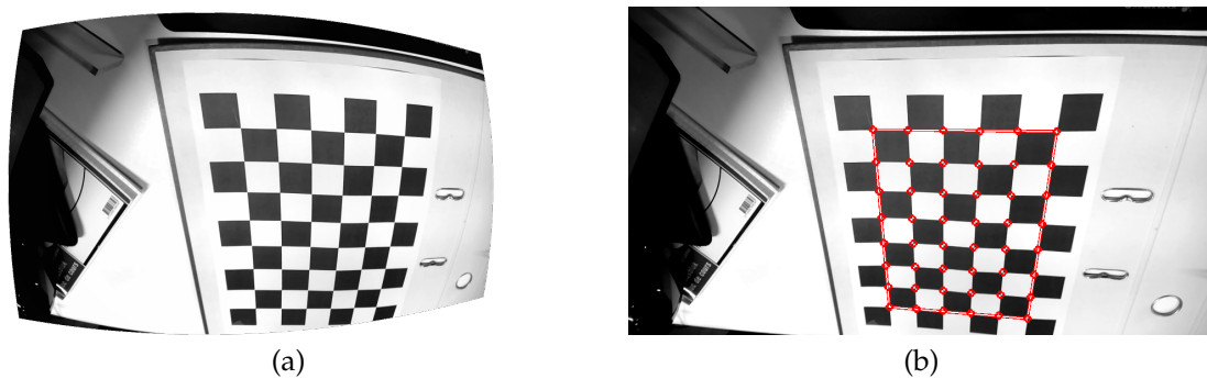
Figure 1. Example of the detection of a checkerboard. A radially distorted input image (a) and the undistorted image with the detected points highlighted in red (b).
