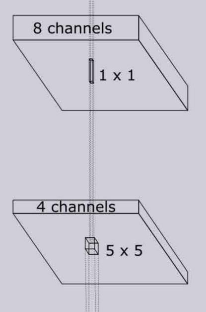
The next two layers transform the lower-level features into high-level colour features using the combination of convolutions and rectified linear units (ReLU's) to good effect.
