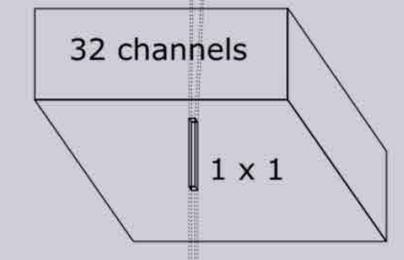
The first layer transforms the RGB input to 32 lower-level features, using a large spatial support.
