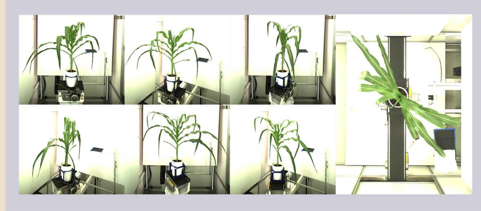
The camera input from the PHENOVISION system comprises 180° views and a top view of the object maize plant. Because of the enormous volume of data, we require a fast and accurate 3D reconstruction technique. Voxel carving fits well, but requires segmented input images.
