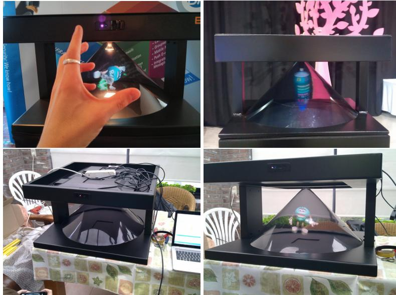
**Figure 6.13:** Two conic 360 degrees displays prototype of size 80 cm  $\times$  80 cm  $\times$  50 cm.
