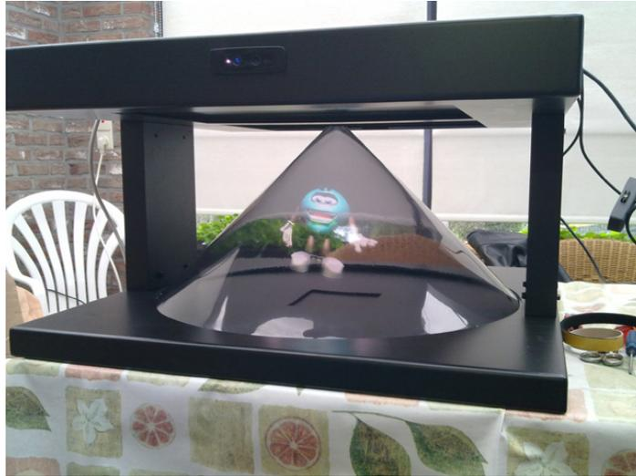
**Figure 6.1:** A see-through display allows multiple users to interact with a virtual object while maintaining eye-contact.
