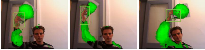
**Figure 5.6:** Context learning allows our hand tracker to automatically learn the appearance of any object that exhibits coherent motion with the hand itself. In this image, the person is holding a magazine.
