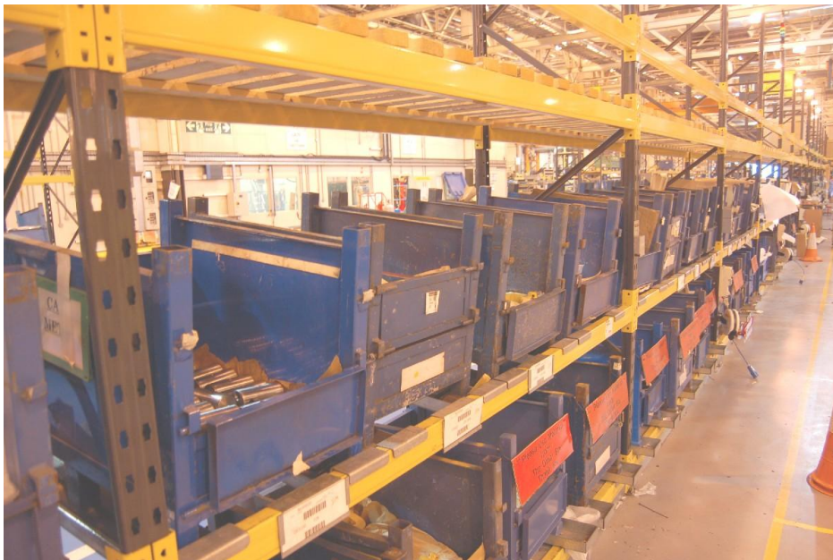
Figure 5.3, Stores situated lineside with two-bin kanban system.
