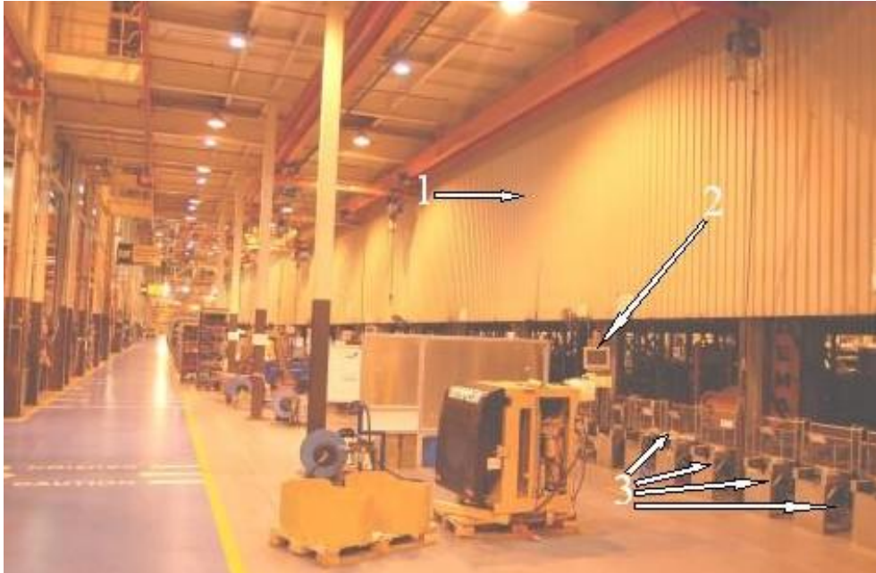
Figure 5.9, Part of the ASRS system. 1. Stores 2. Computer terminal 3. Pick up locations.
