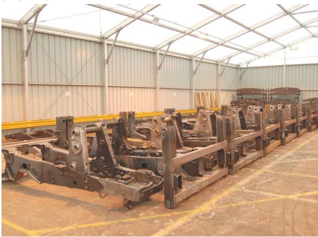
Figure 5.7, BHL frames in sequenced buffer waiting for painting.
