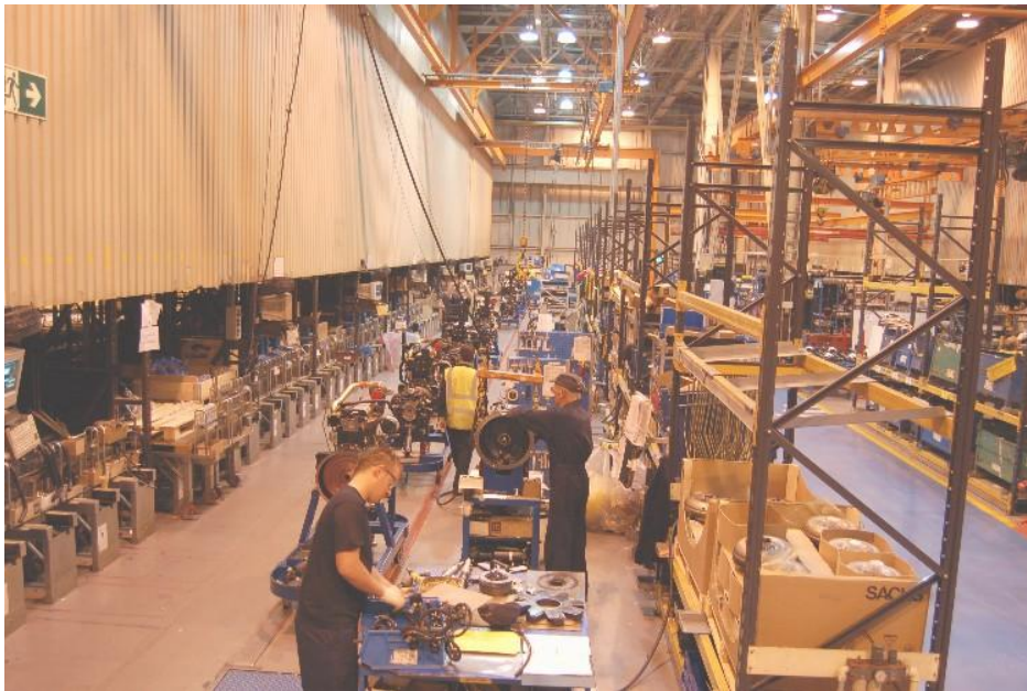
Figure 5.14, Overview of the Engine Subassembly. ASRS , assembly line, stores, from left to right.
