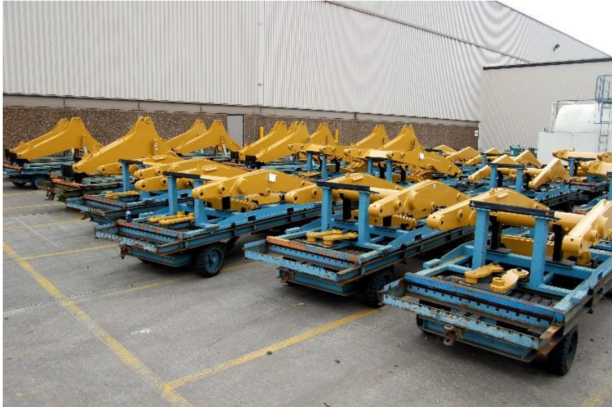
Figure 5.10, BHL booms and loaders waiting in buffer to be transported to POU.
