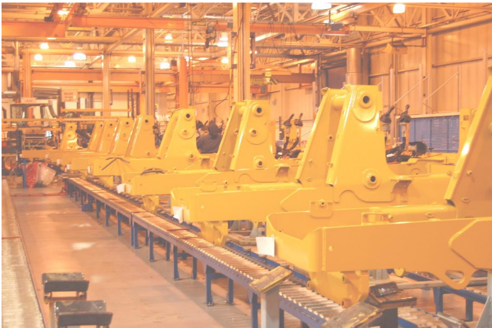
Figure 5.5, Frames (BP1) waiting on rollerbed lineside.
