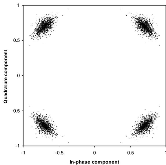
**Fig. 4 : Scatter diagram for  $f_L=0$ ,  $f_H=2.56/T$ ,  $N-1$  disturbing users**
