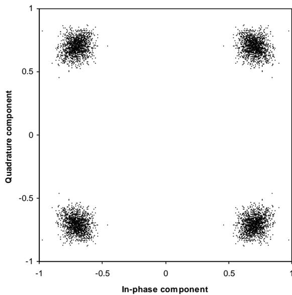
**Fig. 5 : Scatter diagram for  $f_L=2.56/T$ ,  $f_H=5.12/T$ ,  $N-1$  disturbing users**
