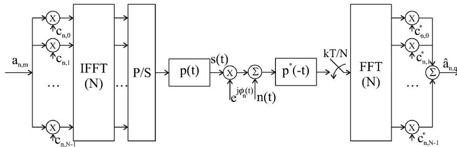
**Fig. 1 : Conceptual block diagram of an OFDM/CDMA transceiver**
