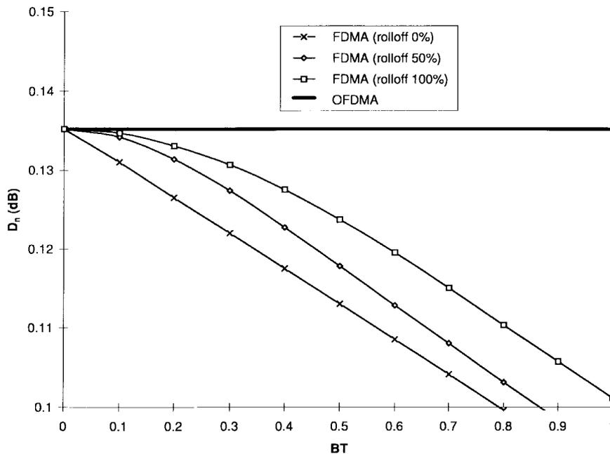
Fig. 4. Comparison of degradations for OFDMA and FDMA.
