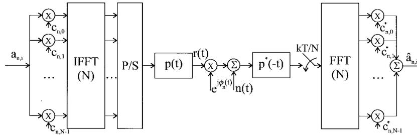
Fig. 1. Conceptual block diagram of an MC/CDMA transceiver for one user.
