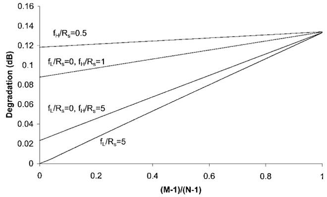
Fig. 2. Degradation as function of  $M$ :  $\sigma_\phi^2 = -40$  dB,  $SNR_{\phi=0} = 25$  dB.
