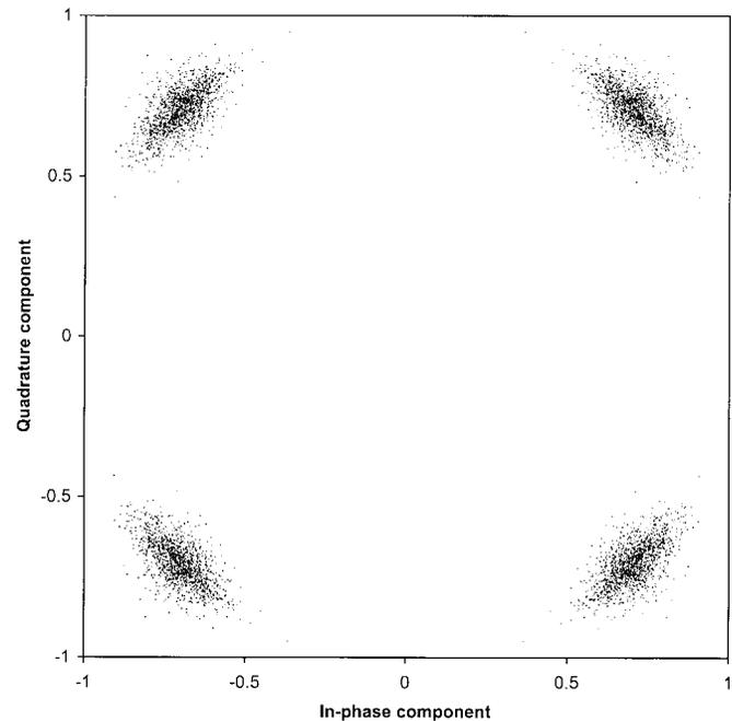
Fig. 3. Scatter diagram for  $f_L = 0$ ,  $f_H = 0.02/T$ ,  $N-1$  disturbing users,  $N = 128$ .
