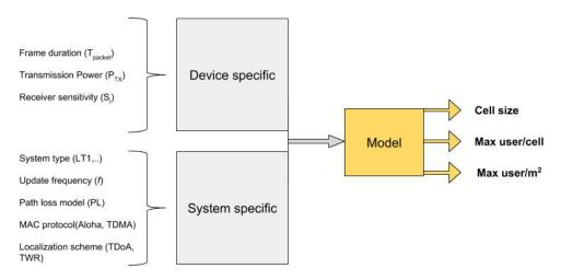
Figure 4. System diagram for UWB indoor scalability model.
