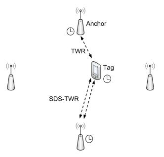
Figure 2. Two Way ranging Scheme.
