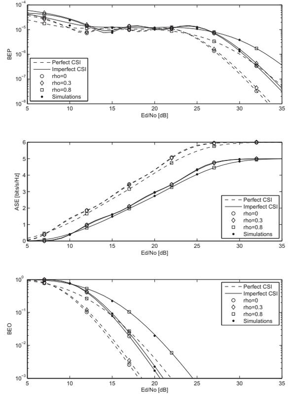
Fig. 3. Average BEP, ASE and BEO of Alamouti's code under correlated Rayleigh fading with  $\rho \in \{0, 0.3, 0.8\}$ , and for perfect and imperfect CSI.
