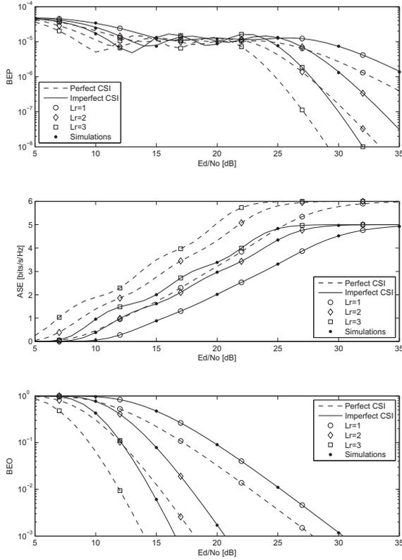
Fig. 2. Average BEP, ASE and BEO of Alamouti's code under i.i.d. Rayleigh fading, for perfect and imperfect CSI, and for  $L_r \in \{1, 2, 3\}$ .
