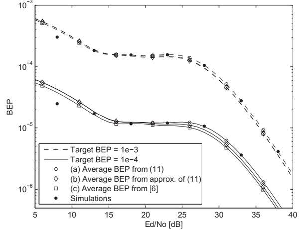
Fig. 1. Average BEP of Alamouti's code under correlated Rayleigh fading, for both a target BEP of  $P_b^* = 10^{-3}$  and  $P_b^* = 10^{-4}$ .
