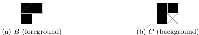
Figure 6.29: Alternative structuring elements for the hit-miss transform for an upper-left corner detection.
