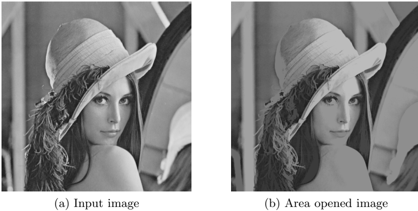
Figure 4.11: Area opening of a greyscale image, with \lambda = 10\,000 .
