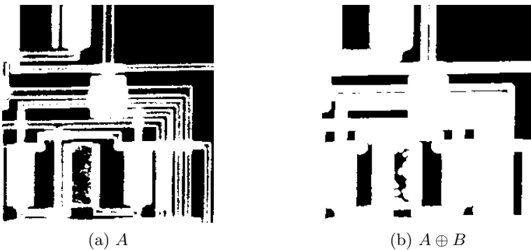
Figure 2.6: Binary dilation by B , with B a disc structuring element. White are object pixels, black is background.
