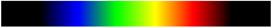
Figure 3.1: The visible spectrum, going from violet (380 nm) to red (780 nm). Neighbouring lower wavelengths are in the ultraviolet range, neighbouring higher wavelengths are in the infrared range.
