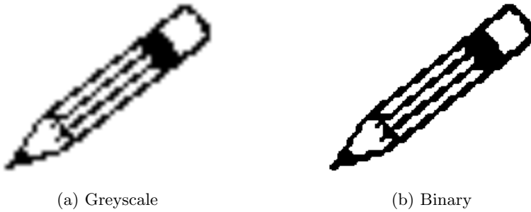
Figure 6.50: A bilinearly interpolated image. Figure (b) is the binary version of figure (a) after Otsu thresholding.
