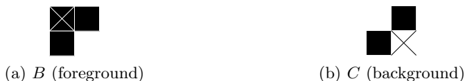
Figure 6.21: Upper-left corner detection with the hit-miss transform. Specific structuring elements are used. The black squares are pixels of the structuring element; the cross is the origin of the structuring element.
