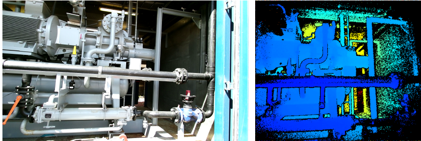
Figure 2.7: Color image (left) and corresponding depth map (right) captured by a Kinect 2 device. Blue pixels in the depth map represent points that are nearby whereas yellow or red pixels denote points that are further away. Missing depth values - represented by black pixels - can occur because the object is either too close or too far away or in case the surface is reflecting too much light.
