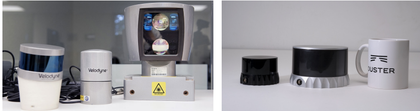
Figure 2.9: Velodyne and Ouster are currently the leading companies developing state-of-the-art 3D scanners based on pulsed lidar technology. Throughout this work, experiments have been conducted with the three different models from Velodyne depicted above, which consist of respectively 16, 32 and 64 lasers.
