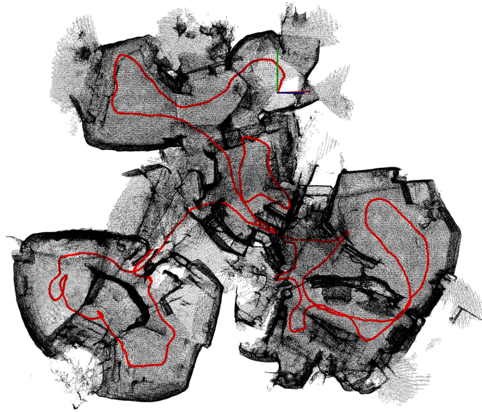
Figure 7.16: Bird's-eye view of the 3D reconstruction of the Sculpture House Gillet in Angleur. The red line represents the trajectory of the lidar scanner.
