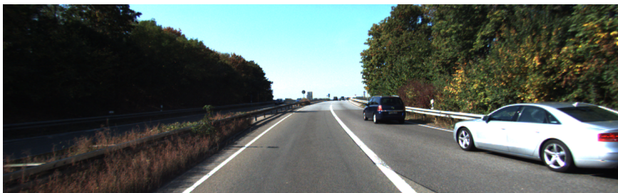
Figure 4.7: Sample image from ‘KITTI01’. The fact that no large buildings are next to the highway, in combination with the high speed of the car and the presence of other moving cars, makes it challenging to correctly estimate the ego-motion of the vehicle.
