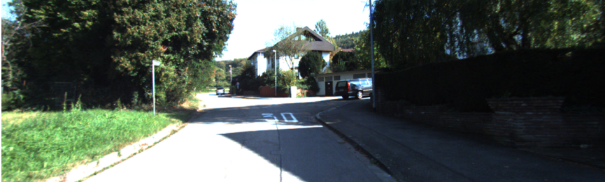
Figure 4.9: Sample image from ‘KITTI03’. The presence of abundance vegetation along the road in countryside areas, makes it difficult to accurately estimate the ego-motion. However, our approach, which favours planar areas, can largely increase the accuracy compared to traditional techniques as it focuses on the more stable regions, such as the (few) buildings that are still present.
