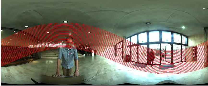
Figure 7.3: The laser points projected on the stitched panoramic image.
