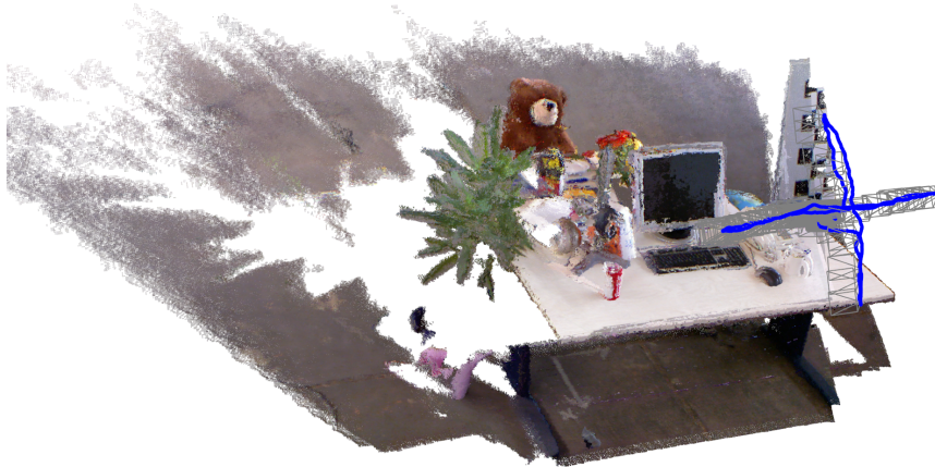
Figure 8.10: The 3D reconstruction and trajectory (in blue) obtained by our system for the sequence fr2_xyz from the RGBD-SLAM benchmark presented in [Sturm 12].
