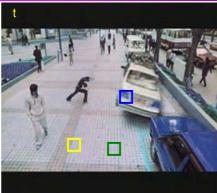
In uniform regions (green squares) motion cannot be accurately estimated Along edges (yellow boxes) motion reliability is also low, unless motion is perpendicular to the edge
