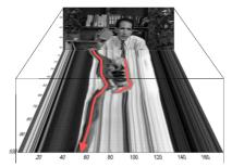
Advanced temporal filters for video filter along the estimated motion trajectory – this is called motion compensated filtering
