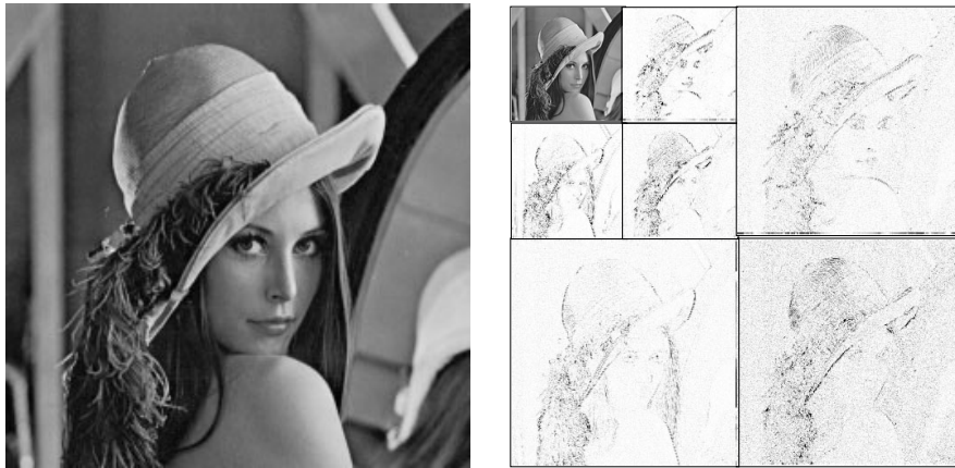
Figure 2.6: An image (a) and its 2D DWT (b). Black pixels denote large magnitude wavelet coefficients.
