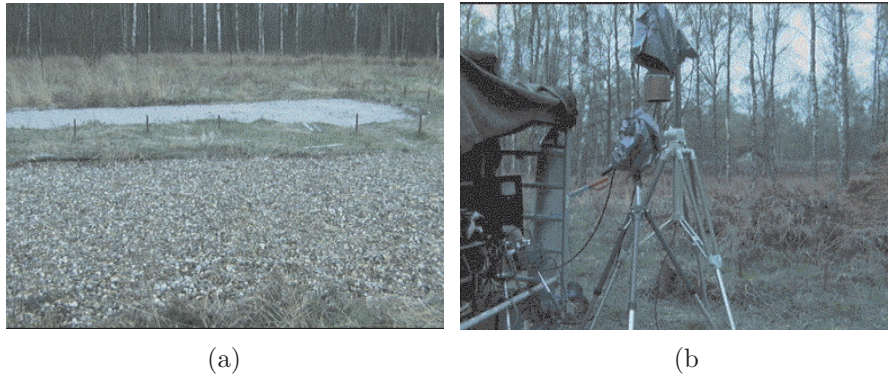
Figure 6.3: Acquisition of a data set of IR images of landmines. (a) Dummy minefields and (b) a test setup with two IR cameras.
