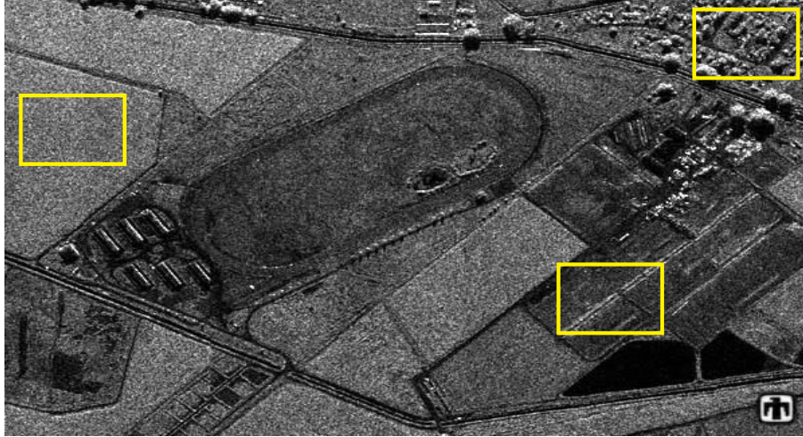
Figure 5.27: A SAR image and an illustration of a homogeneous, an edged and a highly heterogeneous region. Typical speckle filtering methods apply different types of filtering in these regions.
