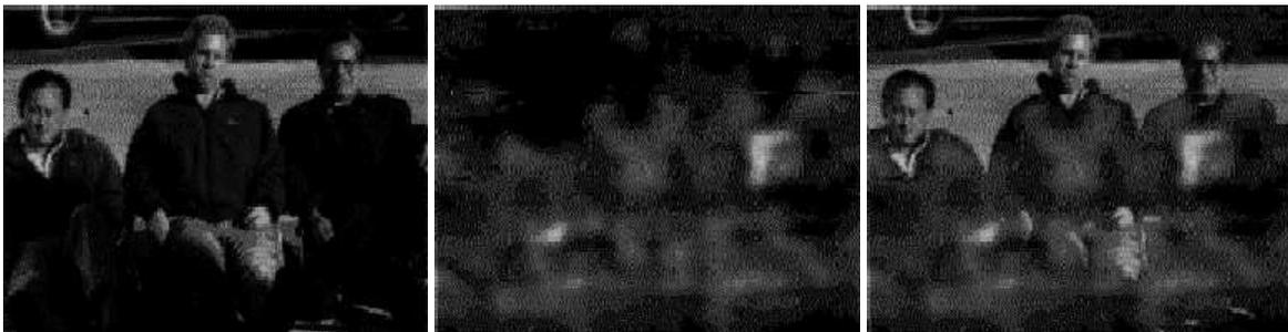
(a). Image 1 (Visual)    (b). Image 2 (Radiometric)    (c). Fused image \*
