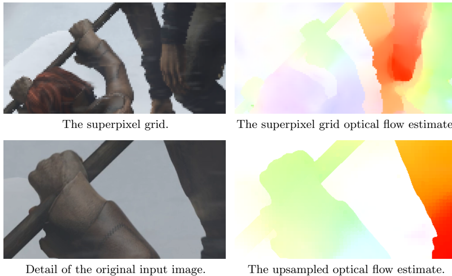
Fig. 9. Illustration of the proposed method: the superpixel grids (top left) for both input images are processed by a dense pixel-based method, resulting in an optical flow estimate for the superpixel grids (top right). After upsampling (bottom right), we arrive at an optical flow estimate for the original input image (bottom left).
