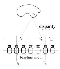
**Fig. 1**: The central camera and the reference camera observe the same point P at  $x_1$  and  $x_2$ . The orthogonal distance from the baseline to point P can be calculated when the baseline width, disparity and focal distance of the cameras are known.
