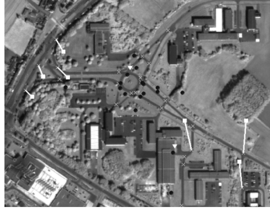
Figure 6. Matching result using relaxation labeling. (square=correct, circle=null, triangle= wrong).
