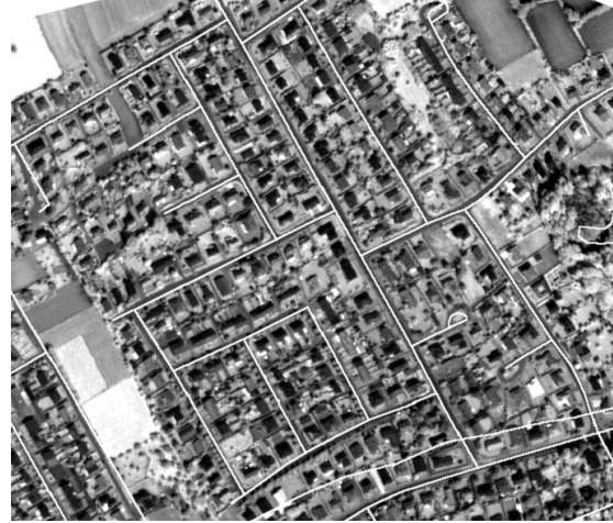
Figure 4. Result of registration process using rubbersheeting transformation.
