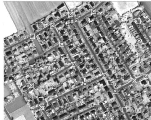
Figure 2. Detection of junctions. Crosses are junctions after verification
